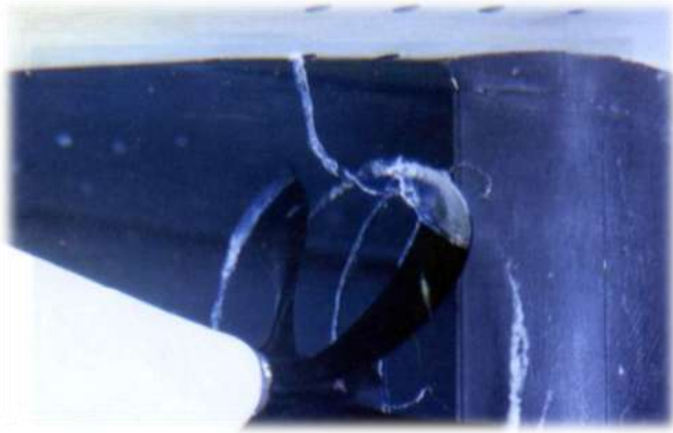
Figure III.6: Cavitation du tourbillon de coque [7]
