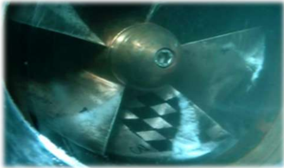
Figure III.3: Cavitation à poche [7]
