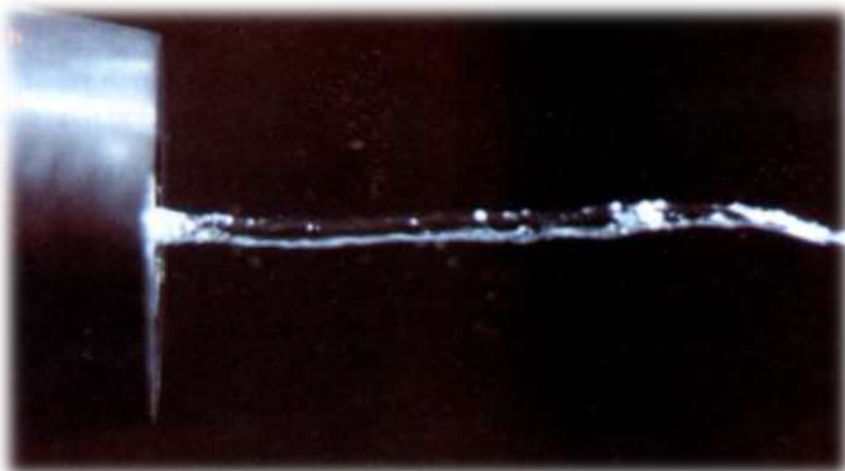
Figure III.5: Cavitation du tourbillon d'ogive [7]
