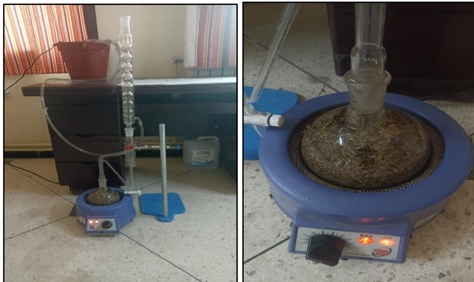
Figure 41. Hydrodistillation protocol using the Clevenger Apparatus Method ( Original picture )
