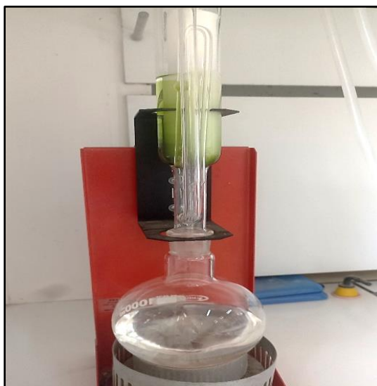
Figure 42. Vegetable oil extraction using Soxhlet (Original picture)
